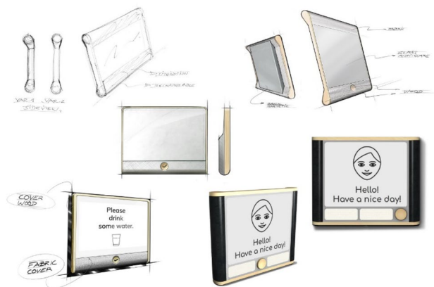
Fig. 6 Design sketches and CAD renderings of the eSticky displays
