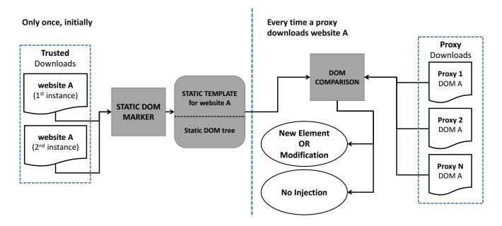
Fig. 1. The methodology followed for detecting content modifications in websites fetched by a proxy. Initially, our framework downloads the target website (or honeysite) multiple times without a proxy, and compares the DOM tree of these downloads, to create a static template of the web page (left). For detecting content modification, it fetches the website through a proxy and compares its DOM tree with the previously generated static template (right).
