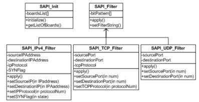
Fig. 5. Simplified UML diagram of the SAPI architecture
