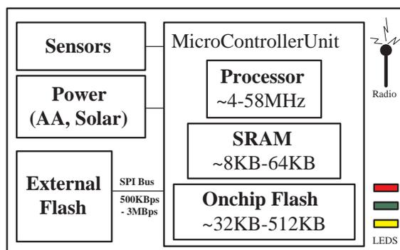
Fig. 1. The Architecture of a typical Wireless Sensor.
