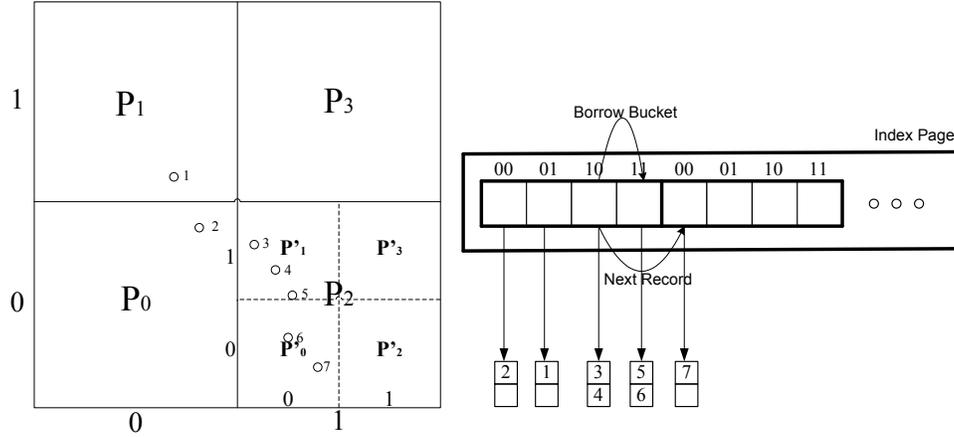
Fig. 10. Creation of a MicroGF Index Page. The two figures show at a high level how the trajectory on the left is encoded into a set of two index records.
