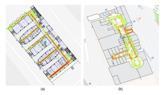
Fig. 8. Wi-Fi datasets. The heatmaps indicate the density of the collected crowdsourced signal strength fingerprints: (a) University of Cyprus Campus and (b) Mall of Cyprus.
