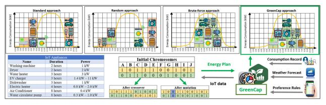
Fig. 4. A daily planning representation of the standard, random, brute-force, and GreenCap methods. The GreenCap is liable to find a sustainable plan for the operation of IoT appliances by only utilizing a Preference Rules (PR) table, a Residential Consumption Record (RCR) history, and a weather forecast. Each IoT device is represented with a letter in the chromosomes stack of the memetic algorithm, and their state is indicated with 1 = ON or 0 = OFF.
