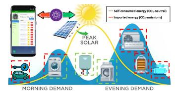
Fig. 1. An energy demand example during a day along with user preference rules and solar energy production. The red dashed lines around the appliances represent the energy used from the grid, and the green dashed lines illustrate the self-consumption of the generated energy from renewable sources.
