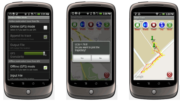
Fig. 2. Screenshots of the SmartTrace demonstration system Left: The configuration panel on the Android-based smartphone client; Middle: A Query Response Message; Right: The matched trajectory displayed using Google Maps.
