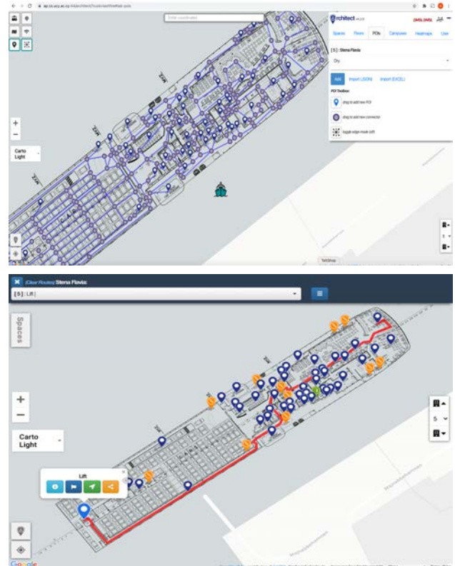
Figure 3: (top) Mapping the ro-ro vessel in our evaluation using our Anyplace Architect tool; (bottom) Obtaining navigation instructions and information search in Anyplace Viewer.
