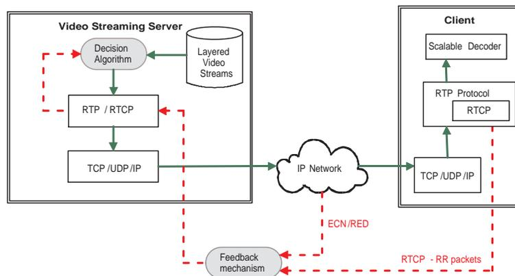
Fig. 1. Adaptive fuzzy-based video streaming architecture.
