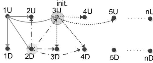
Fig. 5: The event  $E_1 = 3UB \& 2DB$ . Nodes 3U and 2D broadcast the message. Dotted arrows indicate receiving nodes due to 3U broadcasting whereas line dotted arrows indicate receiving nodes due to 2D broadcasting.
