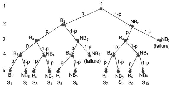
Fig. 1: Probability tree diagram for the case of five nodes.
