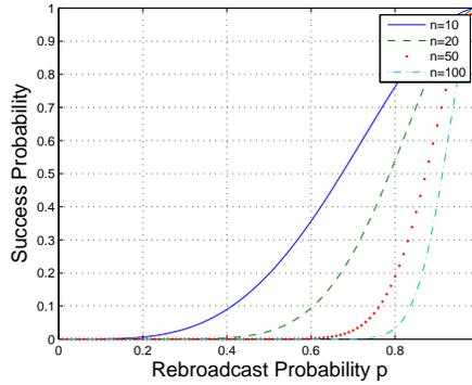
Fig. 3: Probability of all vehicles receiving the critical message versus the rebroadcast probability for different values of  $n$ .
