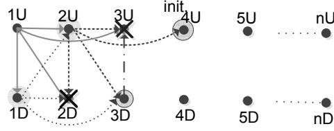
Fig. 9: The event  $E_{4/2} = (2UB \& 1DB) \& (3UNB \& 2DNB)$ . The broadcasting nodes are cycled. 4D is considered to be the initiator node in order to calculate a lower bound on the success probability.
