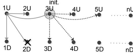
Fig. 6: The event  $E_2 = 3UB \& 2DNB$ . Node 3U broadcasts the message. Dotted arrows indicate receiving nodes due to 3U broadcasting.
