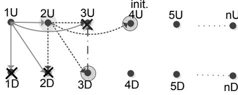
Fig. 8: The event  $E_{4/1} = (2UB \& 1DNB) \& (3UNB \& 2DNB)$ . The broadcasting nodes are cycled. 4D is considered to be the initiator node in order to calculate a lower bound on the success probability.
