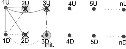
Fig. 10: The event  $E_{4/3} = (2UNB \& 1DB) \& (3UNB \& 2DNB)$ . The broadcasting nodes are cycled. 4D is considered to be the initiator node in order to calculate a lower bound on the success probability.
