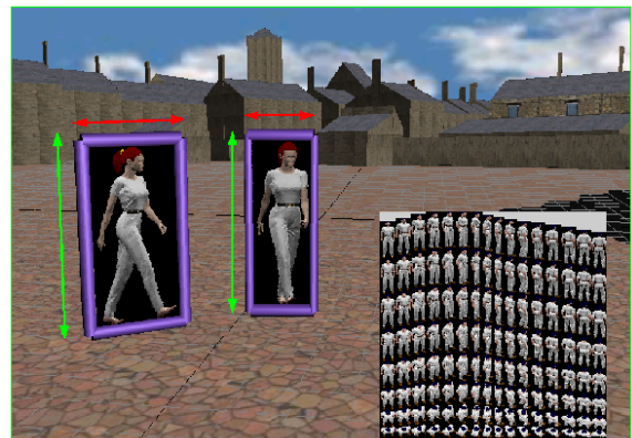
Figure 5: Illustration of the rendering of impostors using a compressed texture. On the bottom right, texture after compression. The images are packed occupying only one fourth of the previous texture as shown in Fig. 4.
