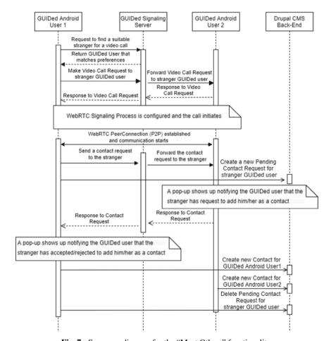
Fig. 7. Sequence diagram for the "Meet Others" functionality.
