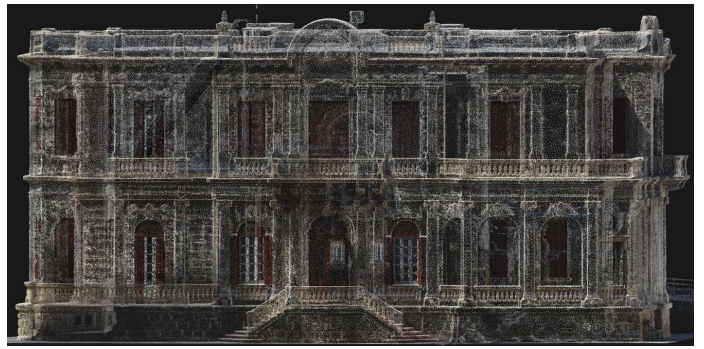
Fig. 2. Sparse Point Cloud of the Pilavakis Mansion
