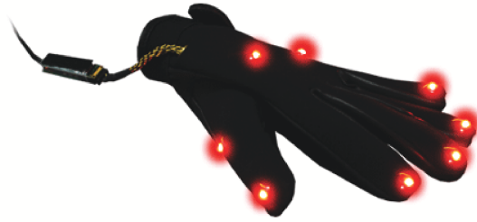
Figure 5.1.: The impulse glove designed by PhaseSpace for real-time finger-tracking solutions.
