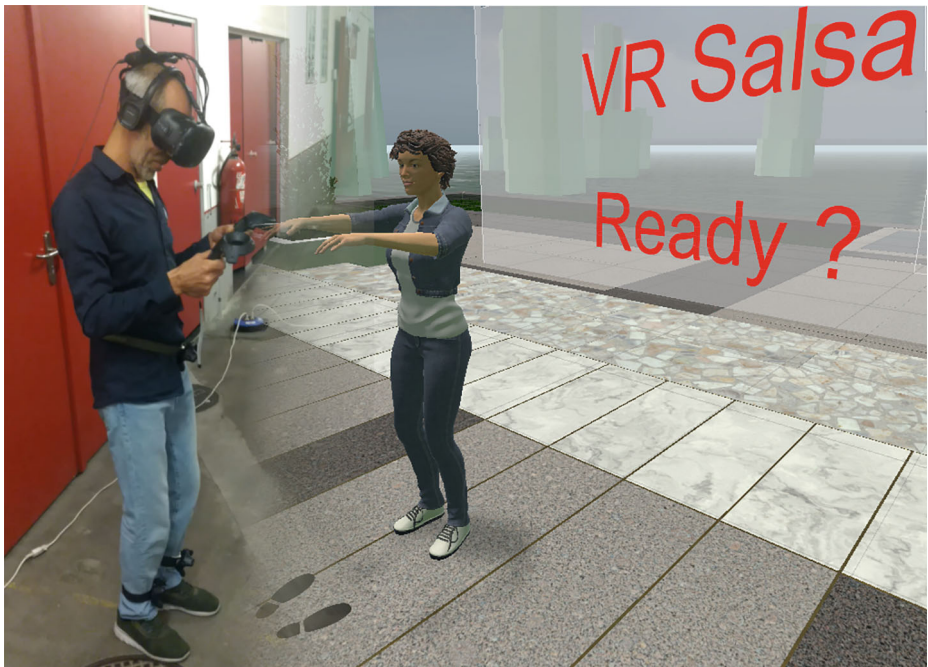
Fig. 1 Our learning salsa gamified VR application. The user wears a virtual reality headset and interacts, in real-time, with a virtual partner using hand controllers. The images of the user in the real-world (left side) and the dancer in the virtual environment (right side) are blended
