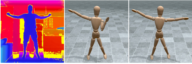
Figure 5: Error detection and correction on motion generated from RGB-depth data (left). The original skeleton as returned by the iPi software is shown in the middle, and the right image presents the repaired motion using our method. The context data in this case came from optical motion capture acquisition.
