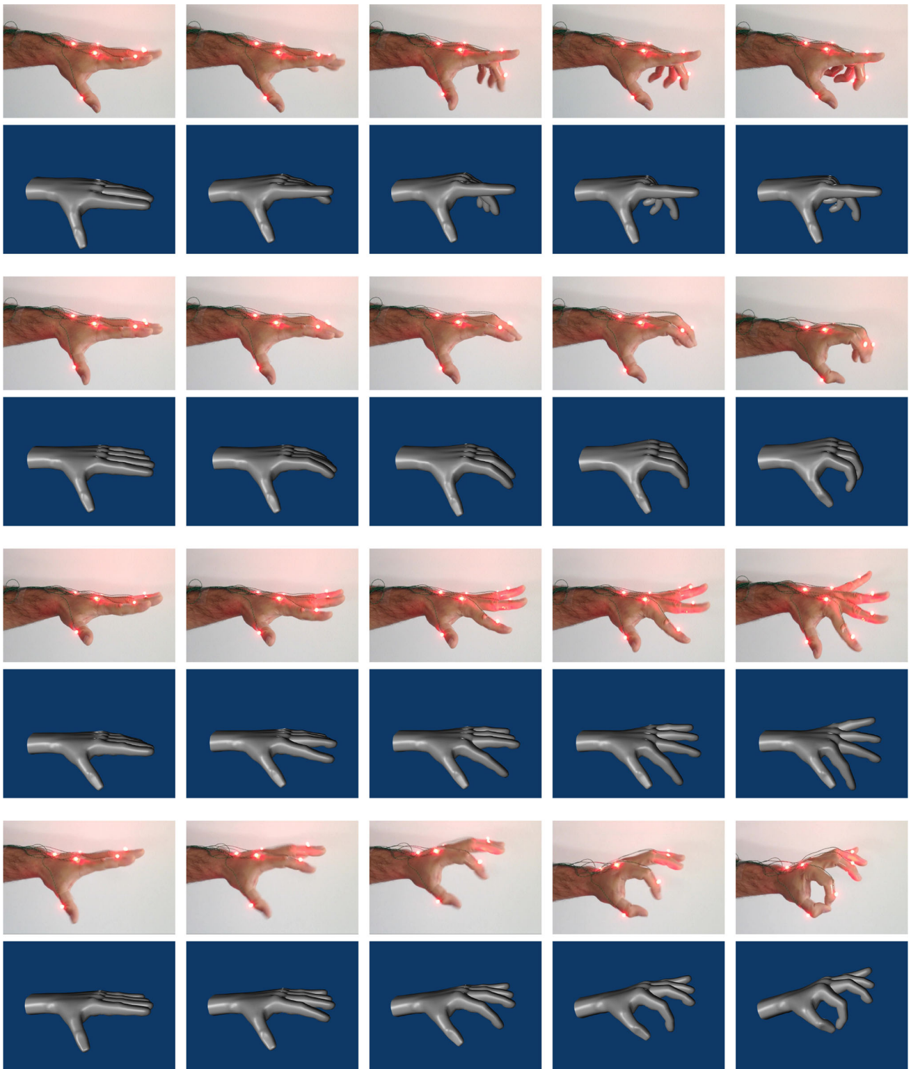
Fig. 12 Four sequences showing examples of hand reconstruction using our methodology at a frame rate of 120 Hz. The first, third, fifth and seventh rows show the true hand posture as recorded using an RGB
