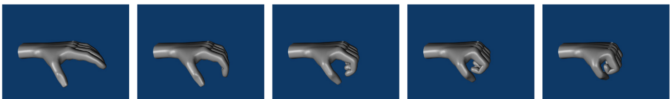
Fig. 14 An example of continuous hand pose tracking; in this example the hand flexes to its ventral side to form a fist
