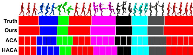
Fig. 13. Comparison of different temporal segmentation methods on motion capture data (subject: 86_03, from the CMU motion capture database). Different colors correspond to distinct actions. The first row illustrates the ground truth classes, the second row shows the segmentation achieved using our method, the third and fourth rows present the results of the ACA and HACA algorithms, respectively [Zhou et al. 2013].
