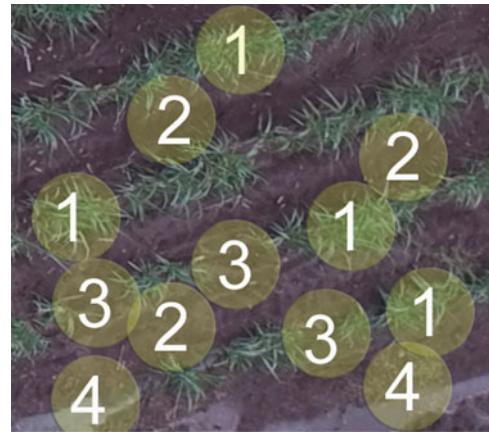
Fig. 2. Identification of missing vegetation from a crop field. Areas labelled as (1) represent examples of sugar cane plants, while areas labelled as (2) constitute examples of soil. Areas labelled as (3) depict missing vegetation examples, i.e. it should have been sugarcane but it is soil. Finally, areas labelled as (4) are examples of 'others', being irrelevant image segments. Colour online.
