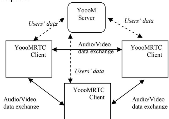
**Figure 2. YooMRTC Module Architecture**
