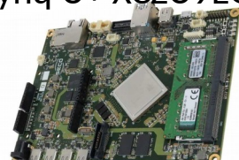
4x Cortex-A53 cores + FPGA (64-bit platforms)
