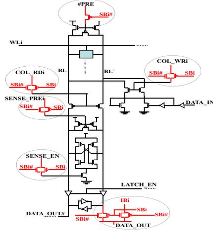
Fig. 4. The control signals, multiplexer and associated drivers shown for a single cell [11]. The dotted circles show the Same-Bit and the added transistors that are used to control the signals when accessing SCC column. Energy is saved when precharging is disabled in columns and senseamps. Also, not driving data during write to SCC column saves energy.
