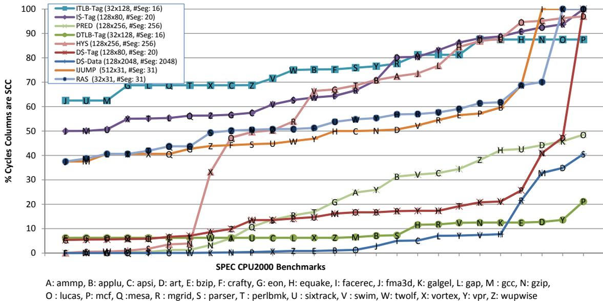
Fig. 1. Frequency of SCC-column for various Benchmarks and Arrays
