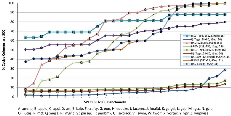
Fig. 5. Percentage of Cycles Columns are SCC as detected by Interval Based Scheme
