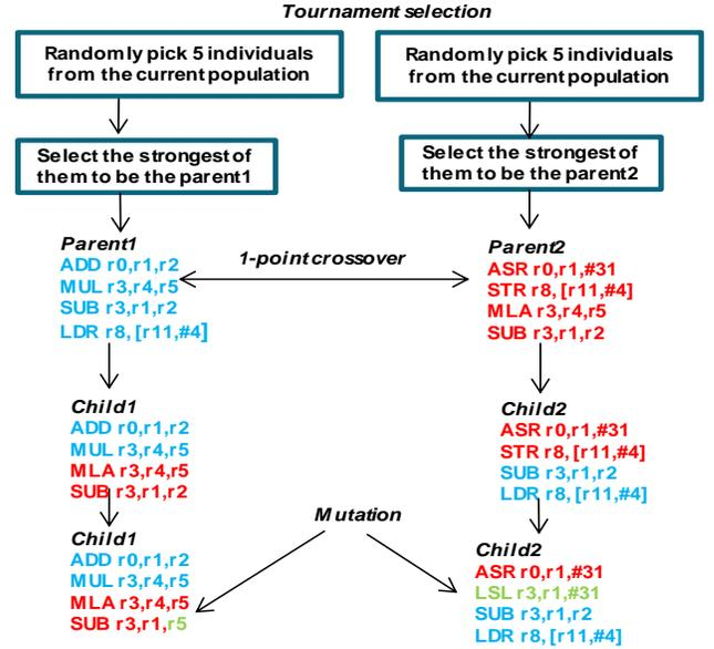
Figure 3. Demonstration of GA operators.
