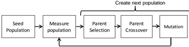
Figure 2. A typical GA flow.
