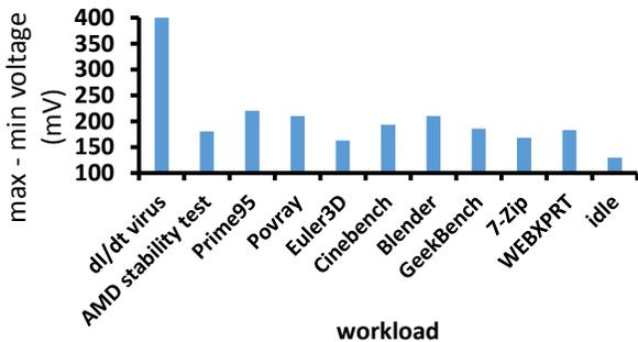
**Figure 8. Voltage-noise results on AMD Athlon CPU.**
