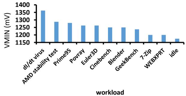
**Figure 9.  $V_{MIN}$  results on AMD Athlon CPU.**
