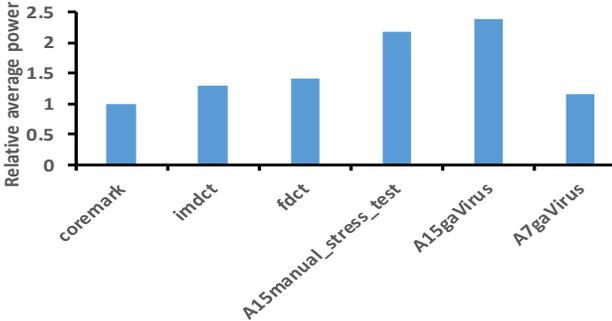
**Figure 5. Cortex-A15 power results.**
