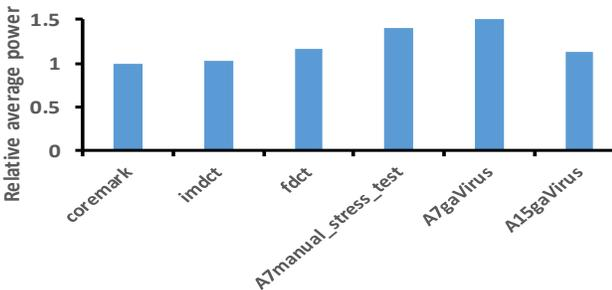
**Figure 6. Cortex-A7 power results.**
